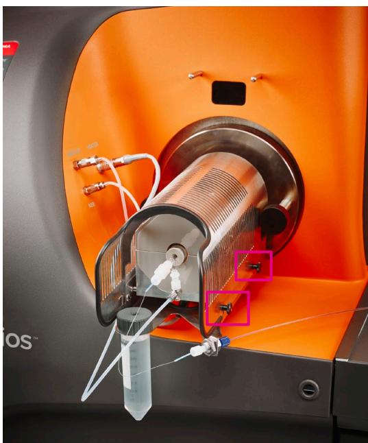
Figure 9. The heat shield on the Helios heater box. There are 4 screws, 2 on each side of the shield, that must be tightened before replacing the shield.
